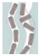
The StabiliTrak Electronic Stability Control System helps you stay the course by detecting the difference between the steering wheel angle and the direction the vehicle is actually turning. It then uses the brakes and, if necessary, adjusts engine torque to help you keep your vehicle on your desired track.
