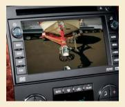
AN AVAILABLE REARVIEW CAMERA SYSTEM<sup>6</sup> helps the driver see certain stationary obstacles on the navigation screen (shown) or rearview mirror while moving in reverse at low speeds.
