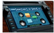
INSIDE TAHOE HYBRID, a power flow diagram on the navigation radio<sup>5</sup> screen informs the driver of how the hybrid system is currently functioning.
